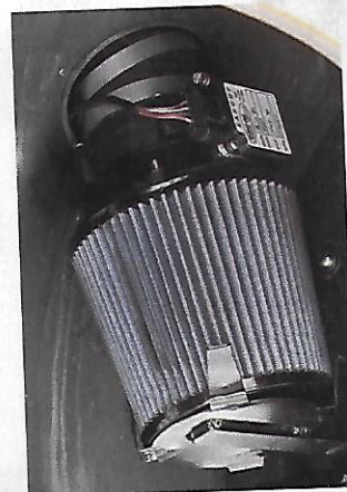
04] Sanchez located the new Pro-M MAF meter and its air cleaner in the wheelwell where it always receives cool air. "The Pro-M MAF is designed and calibrated to mount directly to the air filter the unit is supplied with. Don't separate the parts or you will ruin the application."
