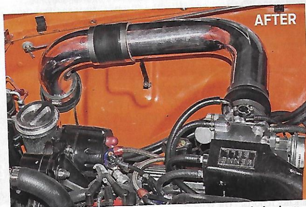
02] Sanchez re-engineered the intake ducting using 3.5-inch aluminum tubing. "I used two prebent 90-degree elbows with a generous curved radius, a hump-hose to allow flex at the engine/throttle-body end, and short lengths of straight hose between the two duct sections and at the MAF end."
