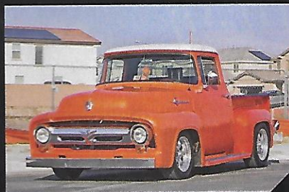
Beneath the sheetmetal is a blown EFI 302, a 4R70W auto trans, and a C4 Vette IRS. The combo wouldn't idle or run smoothly down low.
