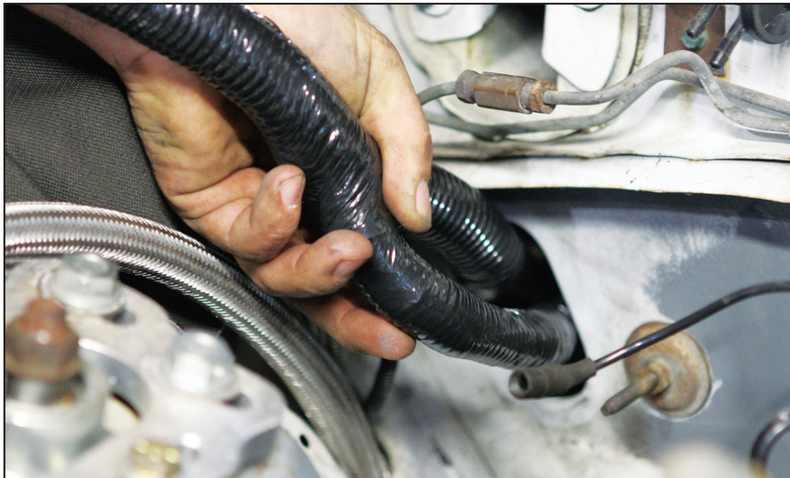
>> Pro-M Racing supplies a brand new wiring harness and it is configured to fit in a Fox-body without any issues—including going through the firewall with a rubber grommet as it were an OEM harness setup.
