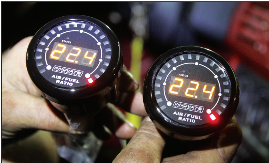
>> A quick download of some Innovate software to your laptop is required to configure the meters properly. There are two gauges included in the kit and we chose to mount them in the glove box away from prying eyes.
