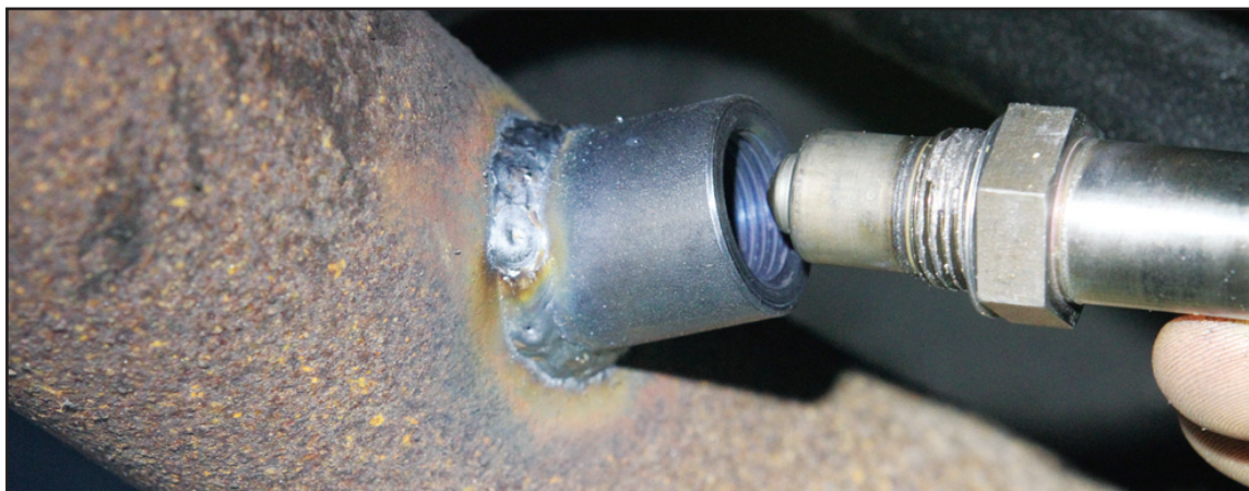
>> The Innovate O2 sensors fit in the stock narrow-band O2 bungs. Unfortunately our no-name brand of headers had the passenger side O2 wedged up against the transmission oil pan. The Innovate sensor wouldn’t fit. Machie fired up the welder and added a bung in a more open space on the header’s collector. This was probably the hardest part of the installation and it wasn’t even Pro-M Racing’s problem but rather our cheap headers.
