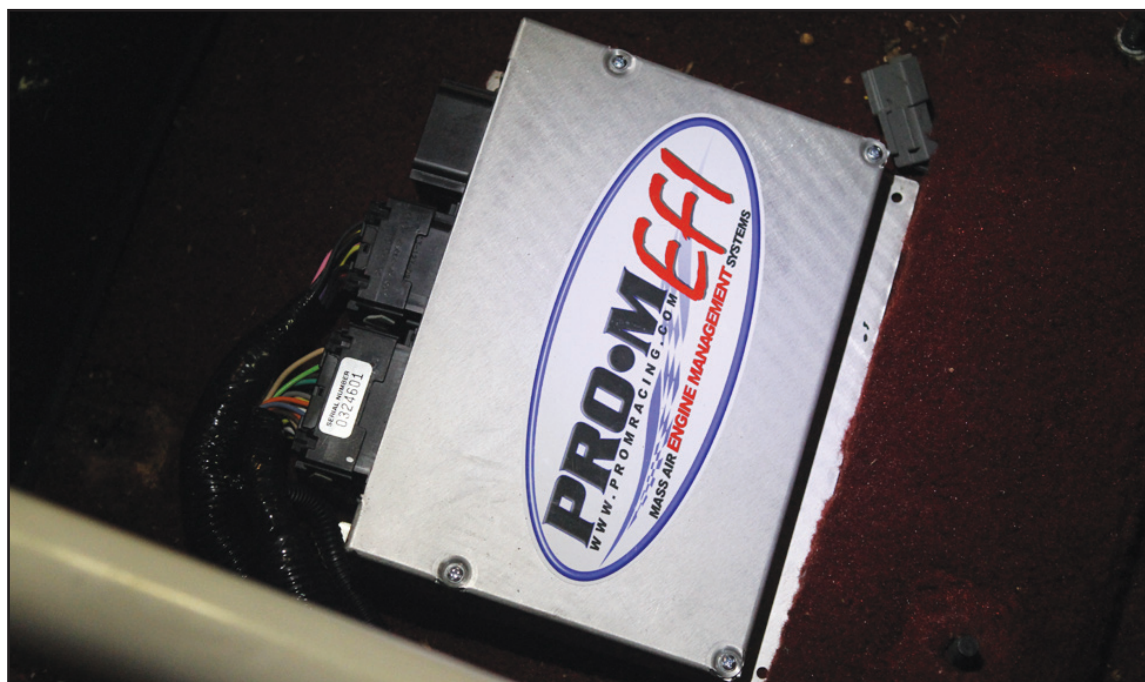
>> The ECU gets bolted to the floor under the passenger seat to keep it out of the way. Its location also has easy access to the OBD-II port so you can hook up the laptop quickly.
