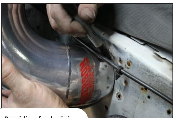
Providing fresh air is an Anderson Ford Motorsport Power Pipe. The inner-fender hole had to be enlarged for the addition of the Power Pipe so Paradise outlined the pipe and made a cut.
