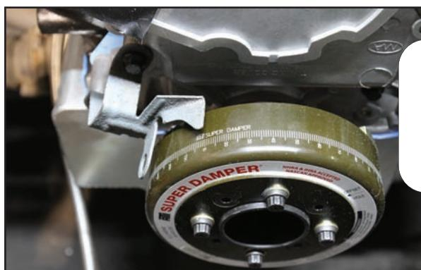
A SFI-certified balancer is required for any vehicle running 10.99 or quicker. It is also helpful to have an excellent damper to eliminate harmful harmonics in our stroker engine. We tapped ATI Performance Products for a 28-ounce Super Damper.
