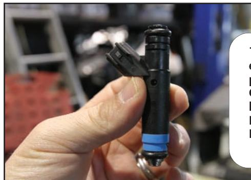
The supercharged 363ci engine gets fed 93-octane pump gas via Ford Racing Cobra Jet fuel injectors (80 lb/hr). We used a set of EV1-to-EV6 adaptors from Ford Racing.
