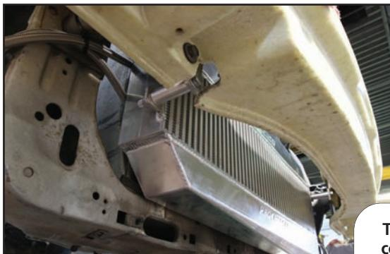
The ProCharger kit comes with an air-to-air intercooler that mounts behind the front bumper. This where experience comes into play, Paradise built new spacers and moved the intercooler rearward to avoid having to cut up the LX front bumper cover.
