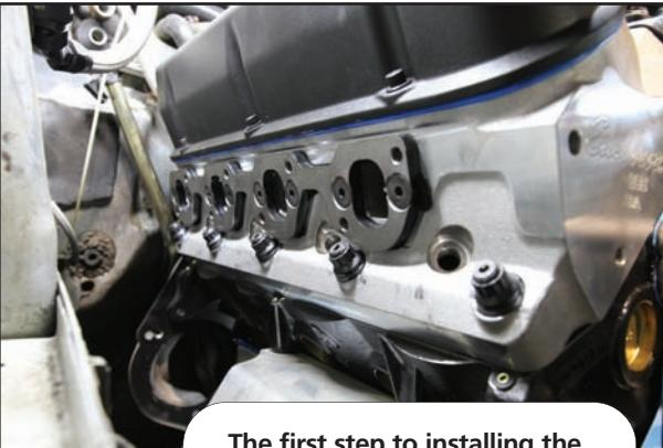
The first step to installing the stainless-steel Kooks long-tube headers was to bolt on the adapter plates for the diagonal bolt-pattern header flanges. The Edelbrock E-205 heads feature a standard header bolt-pattern while the Kooks long-tube headers utilize a diagonal bolt-pattern.
