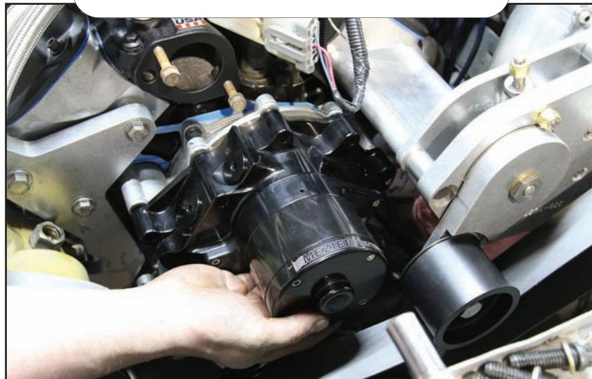
A black Meziere WP312B water pump was selected for its performance first and looks second, though both are equally impressive. The billet water flows 55 gpm, which is what Meziere recommends for supercharged applications.
