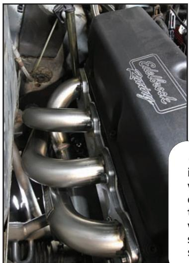
Once the tubes were snaked through into the engine compartment the car was lowered and Paradise bolted each one to the adapter plate. Note the excellent fit on our engine, there weren't any clearance issues with the strut towers, K-member, or even the steering shaft.
