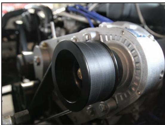
A 3.40-inch upper blower pulley combines with a 7.65-inch crank-pulley to provide our Pony with 13 psi of boost at 5,300 rpm. We expect that boost reading to shoot up to around 16 psi when the engine is singing at its 6,600-rpm redline.
