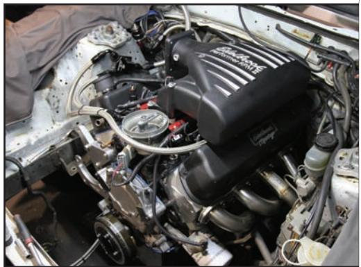
The completed long-block was bolted into the engine bay and then Paradise began bolted on everything else including the ProCharger D-1SC kit, Kooks headers, Meziere water pump, Anderson Ford Motorsport Power Pipe, Pro-M MAF-sensor, Ford Racing Cobra Jet fuel injectors, and Flowmaster exhaust system.
