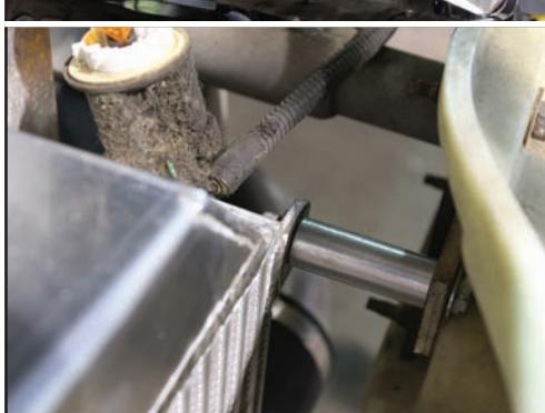
The PA Performance 160 amp alternator mounts easily and cleanly above the relocated Power-Steering pump. We opted for the upgraded Power Wire kit (PN9901) and the black coating to match the rest of our engine.
