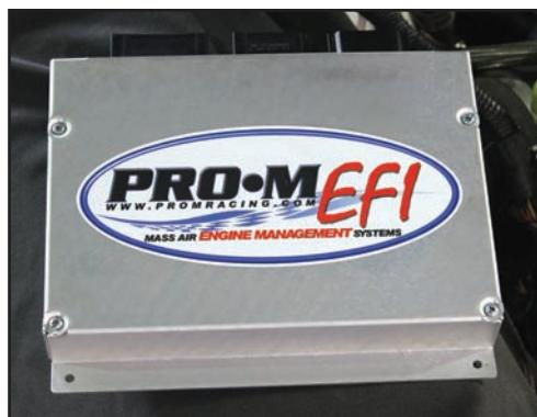
The Pro-M Racing stand-alone EFI system is easy to install and use. Its self-tuning capabilities made our engine swap effortless when it came time to run it on the chassis dyno. Dezotell merely updated the MAF transfer function and fuel injector sizing and the Pro-M ECU did the rest.
